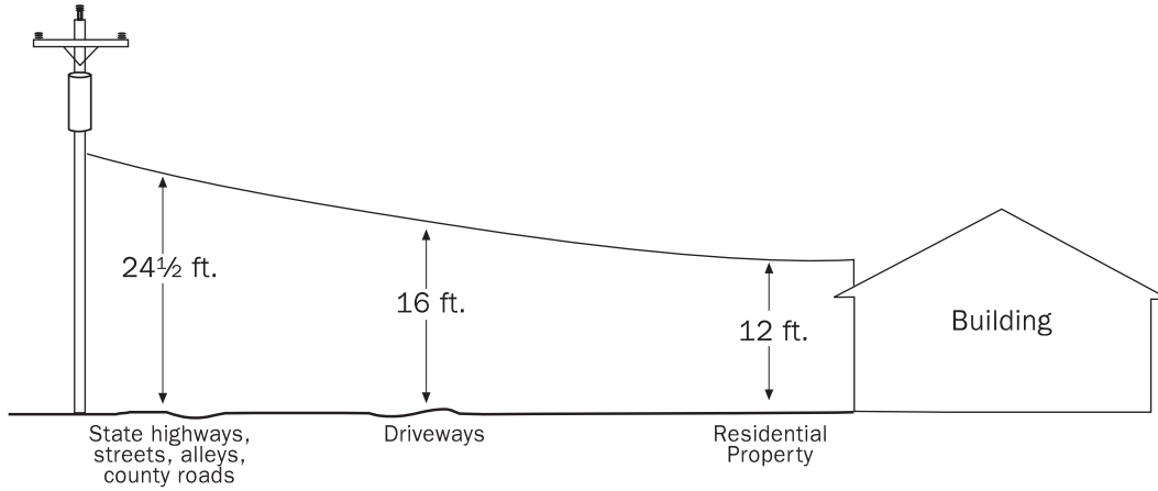
Figure 9. Minimum clearances from ground.
